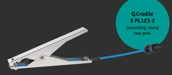
The Q.Crodile X PL123-2 two-pole grounding clamp is particularly suitable for discharging electrostatic charges from potentially charged system parts. Pointed stainless steel teeth penetrate insulating layers such as paint, rust, dirt and grease thanks to high contact pressure. This creates an effective 'metal-to-metal' connection and guarantees reliable grounding. The grounding clamp is intended exclusively for use with the SYMEGA range of grounding systems.
