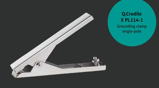
The Q.Crodile X PL114-1 grounding clamp is suitable for all common applications, such as grounding drums, containers and canisters. The robust design of the grounding clamp qualifies it for even the harshest environmental conditions. The stainless steel teeth used are hardened and therefore particularly durable. When not in use, they are protected by the relief holes in the clamp.
