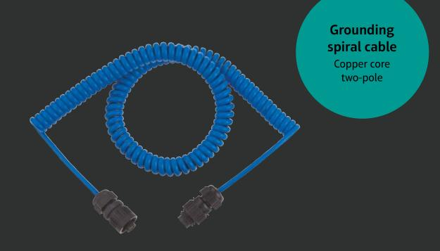
The two-pole spiral cables are used to connect the intrinsically safe circuits of the SYMEGA series grounding monitoring systems with their peripherals (e.g. grounding clamps). The cable sheath is resistant to acids, alkalis, mineral oils, grease and other chemicals. As the spiral cables fulfil all the requirements of the DIN EN 60079-0 and DIN EN 60079-14 standards, they may be used in potentially explosive atmospheres.
